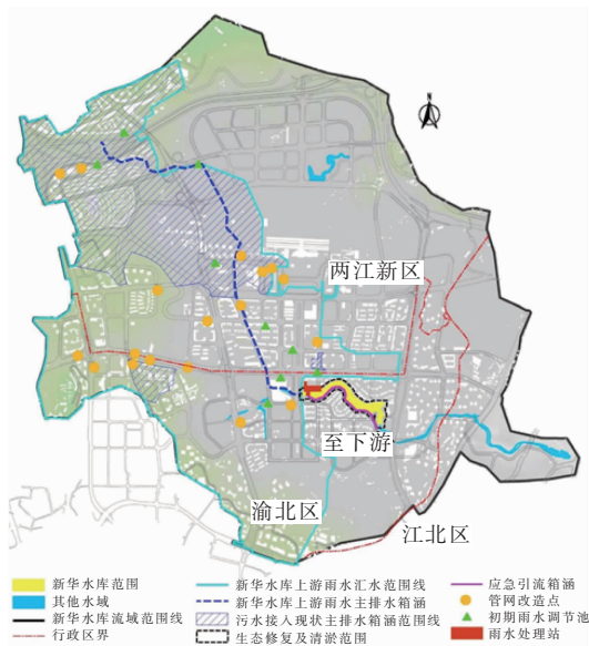
图 3 新华水库流域综合整治措施系统 Fig. 3 Comprehensive treatment measures for Xinhua Reservoir Basin
