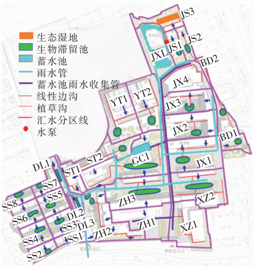
图3 校园海绵设施布局示意 Fig.3 Campus sponge facilities layout diagram
