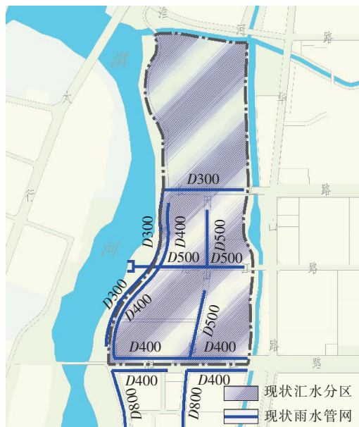
图1 淇水大道易涝区域的现状汇水分区及雨水管网分布 Fig.1 Catchment area and rainwater pipe network distribution map of Qishui Road waterlogging area
