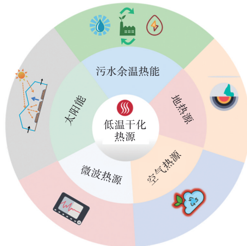
Fig.2 Heat sources for low-temperature sludge drying
