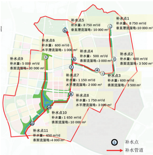
图4 湿地净化系统布置 Fig.4 Layout of wetland purification system
