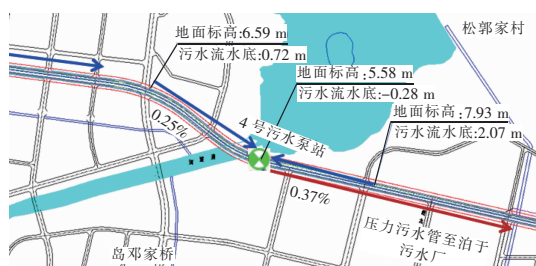
Fig. 3 Analysis chart of rainwater pipeline installed in utility tunnel
