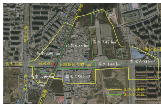
Fig.3 Current situation of concave bridge area drainage system layout
