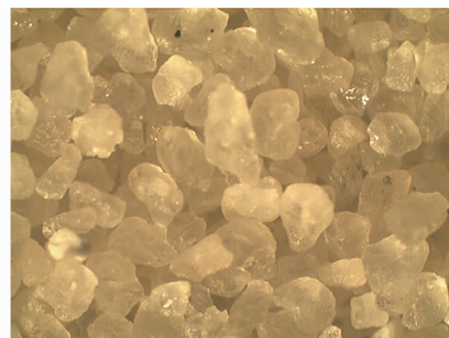
Fig.4 Surface of the sand before entering attrition cell
