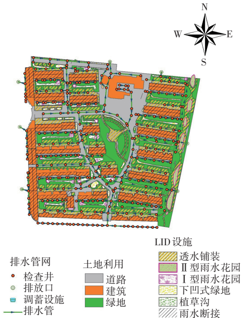
图4 烟波苑 DigitalWater排水模型概化示意 Fig.4 Sketch of DigitalWater drainage model of Yanbo Yuan community
