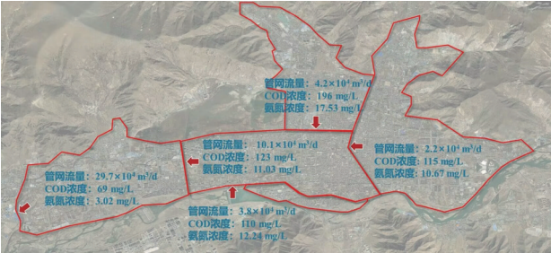
图 6 城区管网沿程水量、水质变化情况 Fig.6 Changes of water volume and water quality along the urban network
