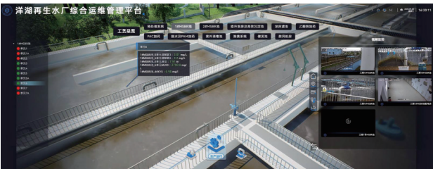
图 14 生产运行模块:工艺段关联实时运行和监控数据 Fig.14 Production operations module:process segment linked with real-time operation and monitoring data
